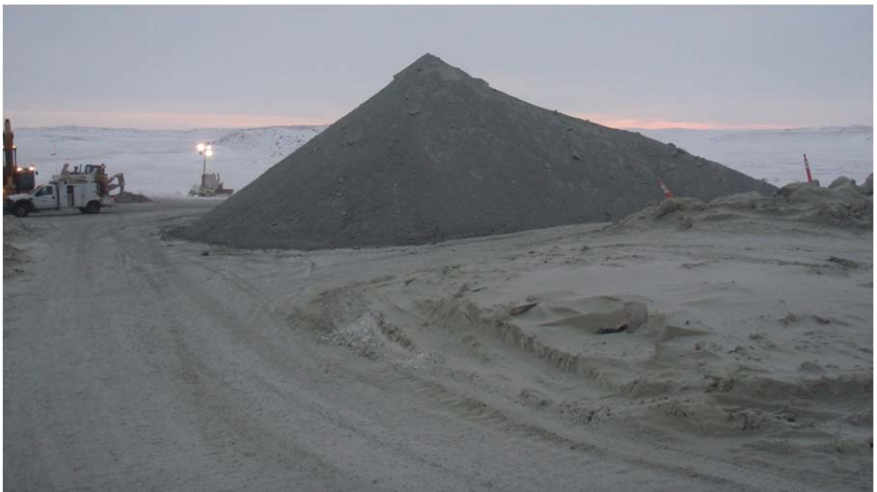
Photo 5 (right): ~ SE view of the front of the FCM stockpile that remains on the FCP Pad after the frozen lumps had been removed/ hauled to the crusher.
